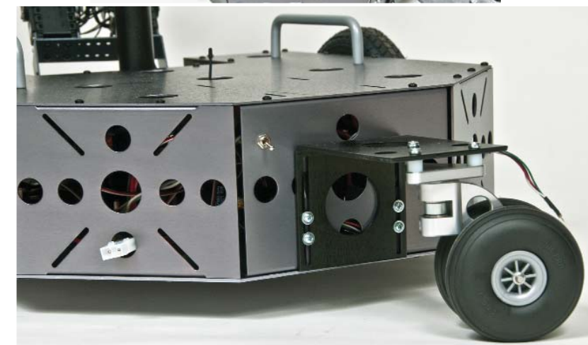
Rear view showing caster kit, power switch, programming and charging cables.
