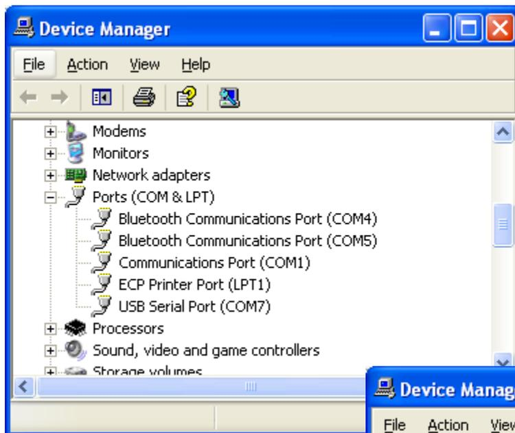
Figure 6: Device Manger with “Ports” Listing Open (USB2Dynamixel Not Connected)
