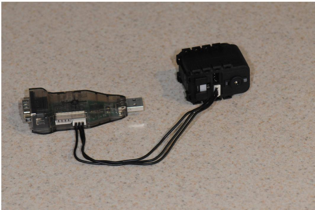
Figure 12: USB2Dynamixel and Servo Connected.
