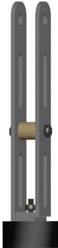
Figure 22 – Completed Lower Leg Assembly
