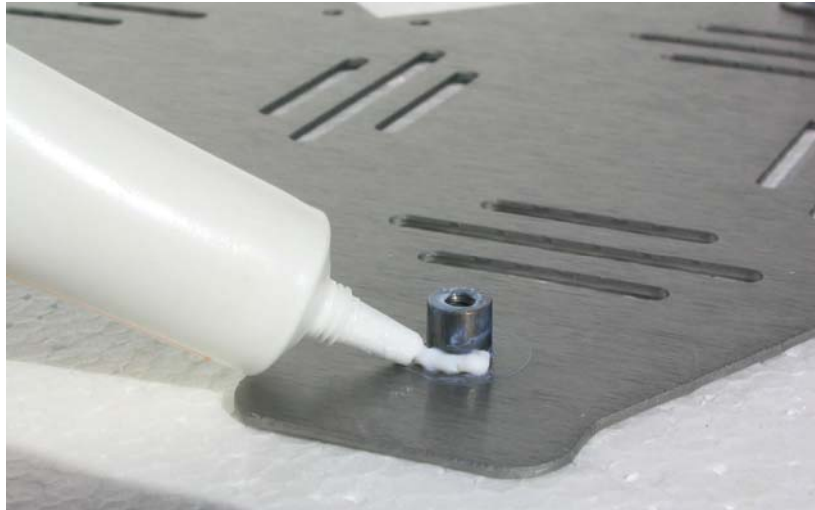
Figure 36: Grease application – Pem Stud
