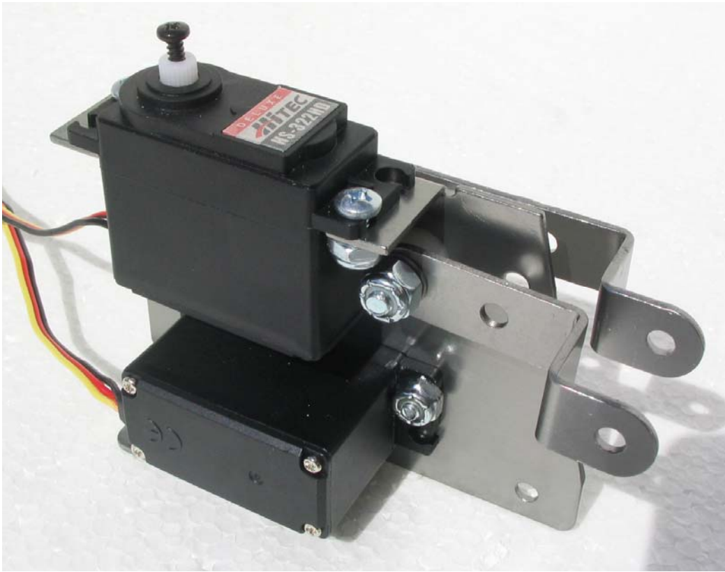
Figure 13 – The Completed Leg Actuator Assembly
