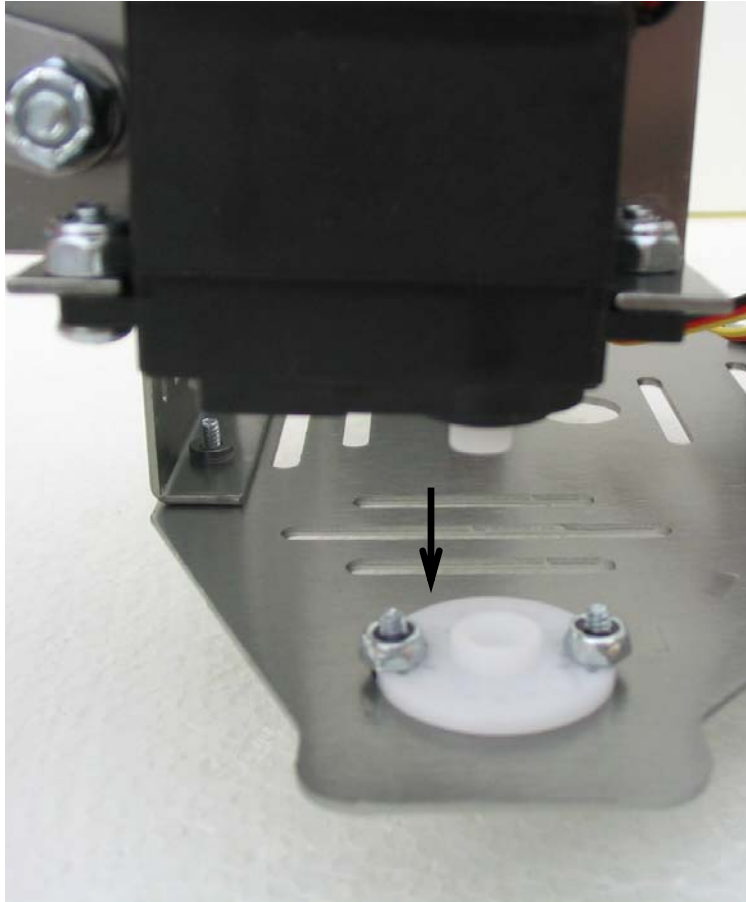
Figure 32: Installing a Completed Leg Assembly
