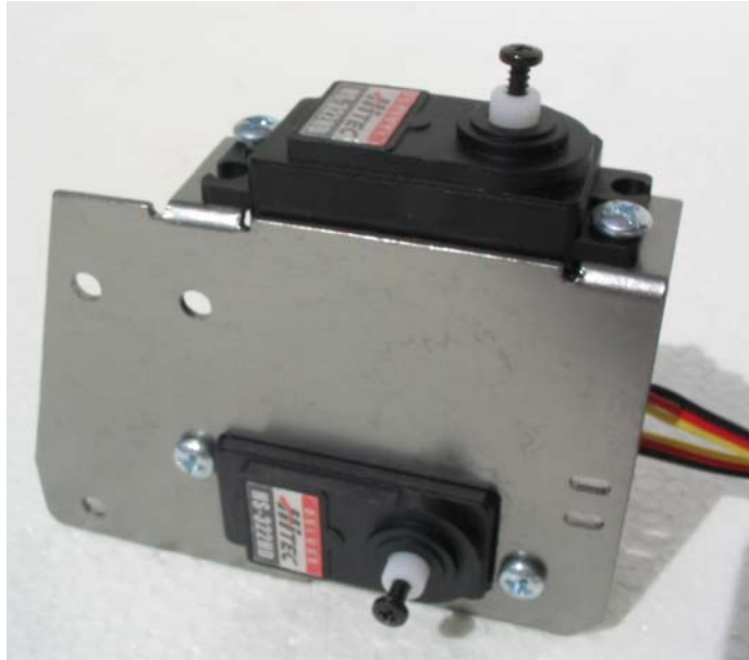
Figure 5: Completed Servo Installation – Front view
