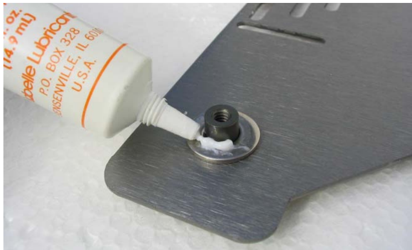
Figure 37: Grease application – SAE Flat washer
