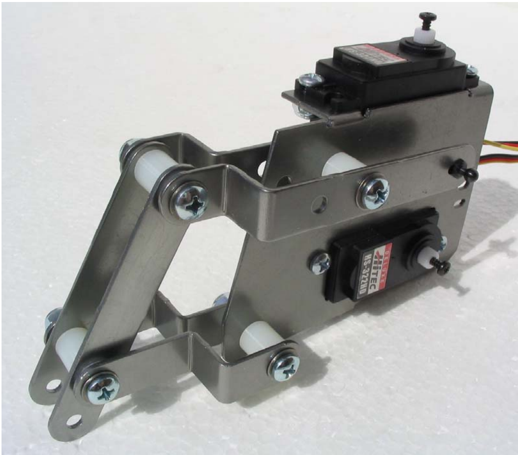
Figure 20: Completed Leg Assembly
