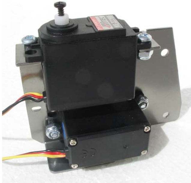
Figure 6: Completed Servo Installation – Rear view
