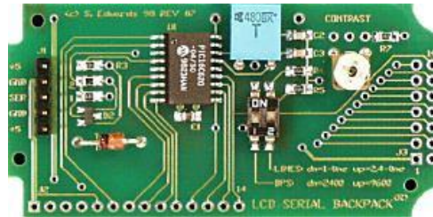
Figure 54 LCD Serial Backpack
